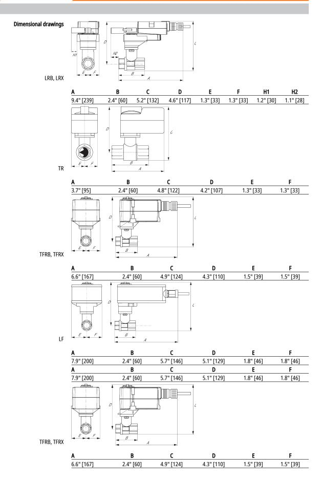
Modulating, Non-Spring Return, 24 V, for DC 2...10 V or 4...20 mA
